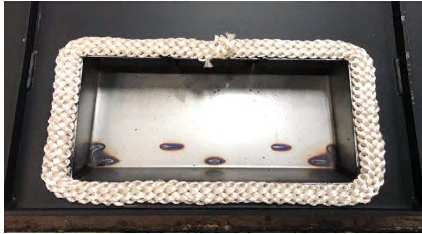
Gasket installed with seam at the back
